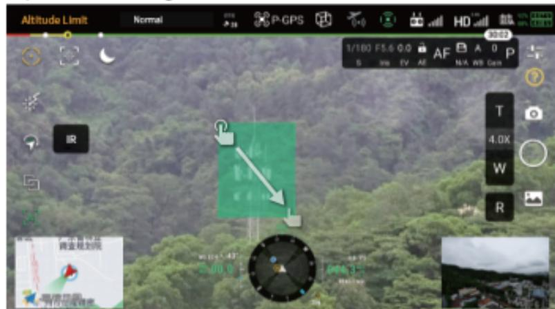
In detection and tracking modes, you can manually draw a box around any target by swiping on the screen. After selecting the target by drawing the box, click inside the box to confirm the selection. If you click outside the box, the tracking will be canceled.
