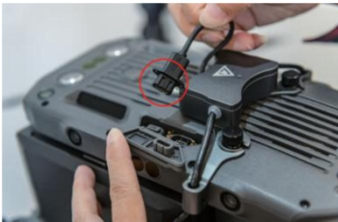
2. Install the red and blue flashing lights in the M300 tripod and connect the light cable with the control box, the installation position and direction as shown:
