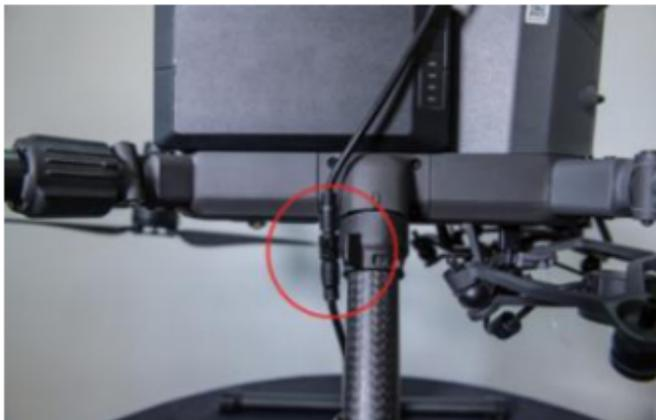
3. Connect the data cable of the control box to the M300, turn on the drone and check the display status of the light on the top of the control box, **if you can see red light of control box on once turning on the drone power, it means the power supply of the OSDK interface is normal.** The next step is to turn on the M300 RTK OSDK function.
